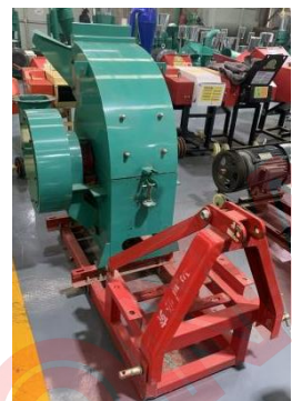
Hammer mill with tractor drive device
