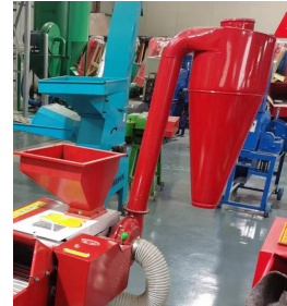
Up inlet for grain milling & cyclone for collect power
